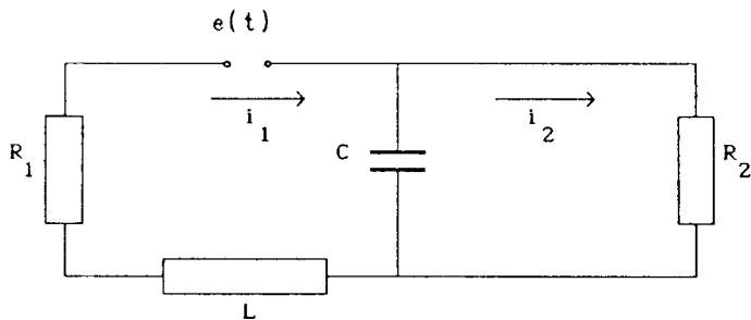
$$R_1 = R_2 = 10 \Omega, \quad L = 1 H, \quad C = 0,01 F.$$
