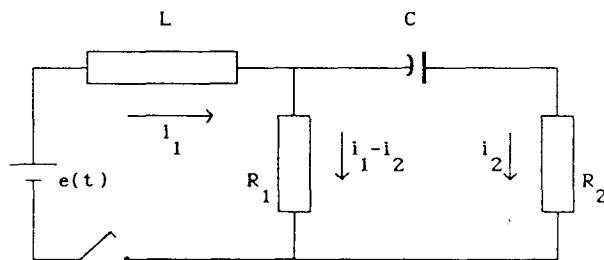
$$\begin{aligned} R_1 &= 200, R_2 = 300, \\ L &= 0,5, e(t) = 50, \\ C &= 50 \cdot 10^{-6}. \end{aligned}$$
