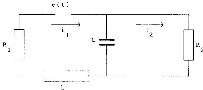
$$R_1 = R_2 = 10 \Omega, \quad L = 1 \text{ H}, \quad C = 0,01 \text{ F}, \quad e(t) = 500\sin 10t \text{ V.}$$
