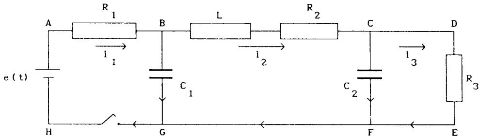
$$R_1 = R_2 = R_3 = 1000, \quad C_1 = C_2 = 20 \cdot 10^{-6}, \quad L = 20, \quad e = 1.$$
